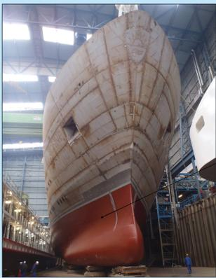
newly developed bow form with 'dent' to prevent 'bubble sweep-down'
